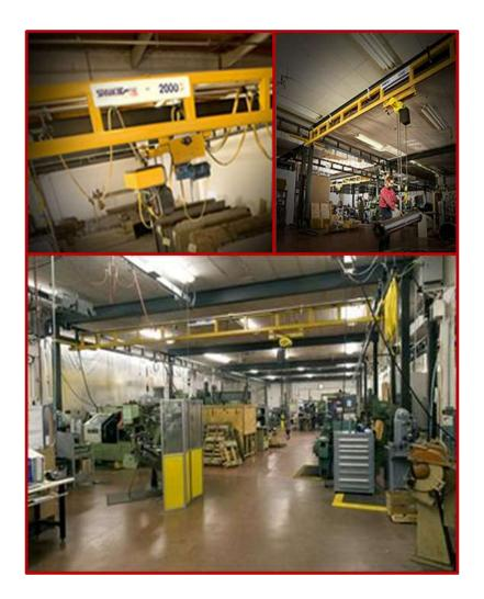
Specifications Floor Space: 800 Sq. Ft Working Height: 19' Bridge Span: 21' Capacity: 1 Ton
